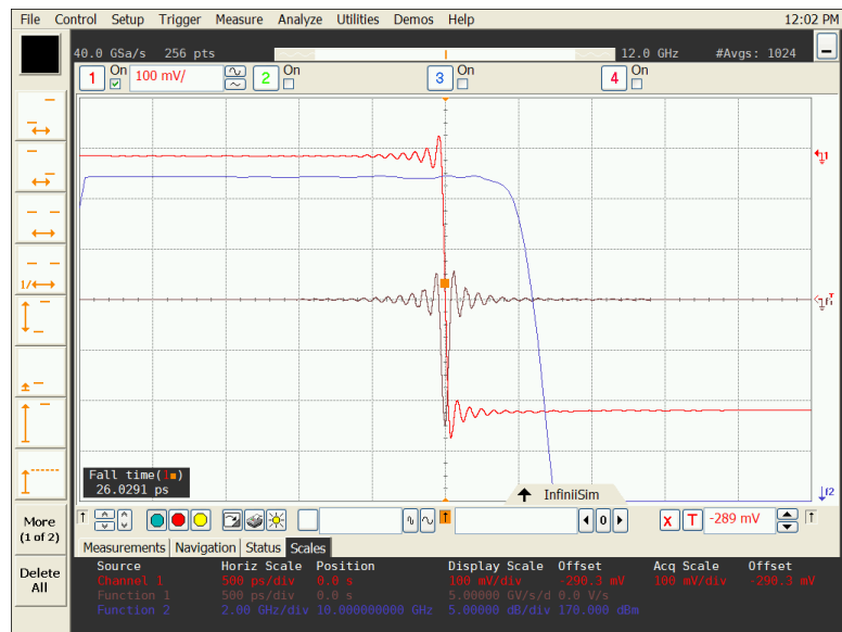
Figure 25. Compensated step response
